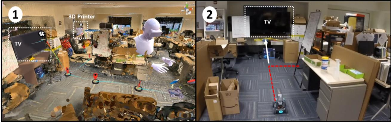
**Fig. 15 Robot IoT Use Case: (1) User specifies the path and authors actions in VR and (b) the physical robot performs the tasks as authored by human in real world.**
