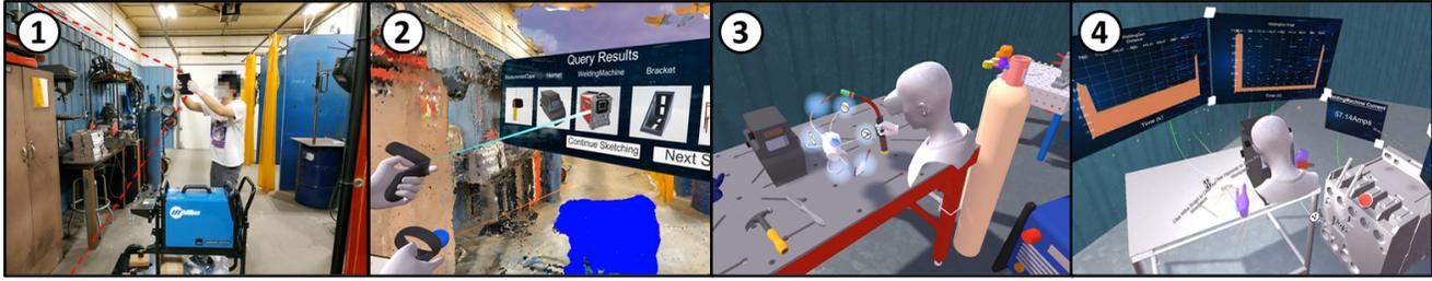
**Fig. 1 Workflow of VRFromX (from left to right). (1) User scans a real environment to get the raw point cloud of the scene using an iPadPro. (2) User creates virtual content by interacting with the point cloud through AI assistance. (3) User attaches real functions to the virtual objects using an Affordance Recommender. (4) User interacts with the reconstructed scene in a virtual environment.**
